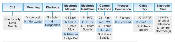
While ordering, specify Process Connection Material, size (Flange or Thread) and Flange rating
